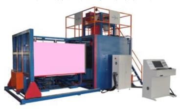
SL-18VF Automatic vacuum foaming machine, adopt batching technology, foaming in vacuum condition. It is composed of storage tanks, batching, mixing, vacuum, mould, and computerized controlling systems. It can be realized numerical control during the whole production. It is used for making all kinds of foam.
