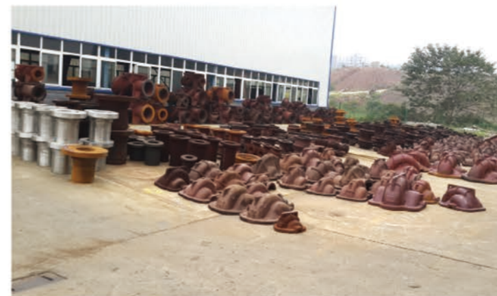
充分的毛坯库存和自然时效，保证了交货的及时性和产品质量的稳定性。 Abundant semi-finished product in store and natural aging make sure the timely delivery and steady product
