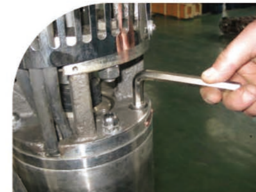
拆卸放气孔丝堵 Disassemble the gas vent plug;
