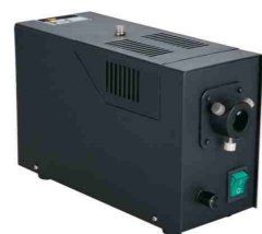
冷光源箱Y3 24V/150W Light source
