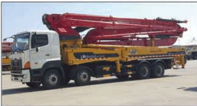
Hold Boom Pump
