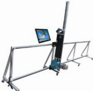
Year 2017, Wuhan HAE developed tablet PC control wireless vertical wall printer
