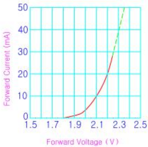
Forward Current Vs. Forward Voltage
