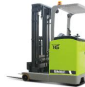
YB16-R1(Standing) Max. lifting height:11,300mm Max. capacity:1,600kg AC Curtis Controller
