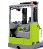
YB20-S1(Sitting) Max. lifting height:11,300mm Max. capacity:2,000kg AC Curtis Controller
