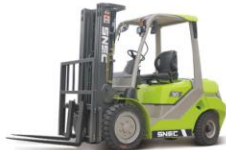
FD30/35-R Diesel Forklifts Max. lifting height:6,000mm Max. capacity:3,000-3,500kg
