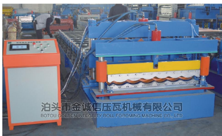
JCX1100琉璃瓦成型机 Glazed Tile Roll Forming Machine
