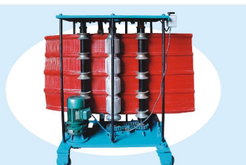
齿形浪板打拱机 Tooth shape corrugated sheet bending machine
