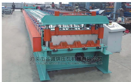
JCX1025楼承板成型设备 Floor Deck Roll Forming Machine
