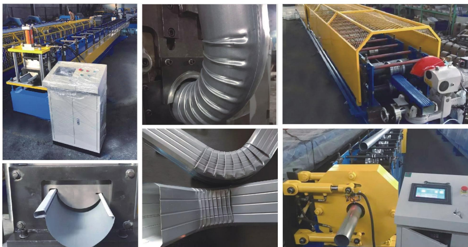
落水管成型设备及弯头机 Forming device for downpipe and bender
