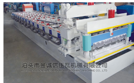
JCX760琉璃瓦成型机 Glazed Tile Roll Forming Machine
