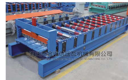
JCX15-225-900彩钢瓦成型机 Color Steel Roll Forming Machine
