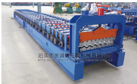
JCX780外墙横板设备 Wall Panel Forming Machine
