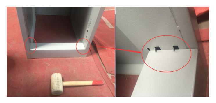
7. Lay down the cabinet and fix the bottom triple shape metal piece with screw.
