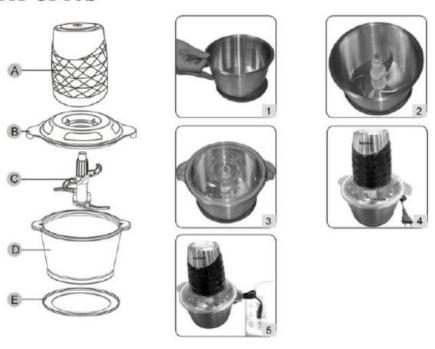
Maximum operating time: 5 cycles (30 seconds on / at least 30 seconds off). After 5 cycles you must leave the appliance to cool down for 10 minutes before its next use.
