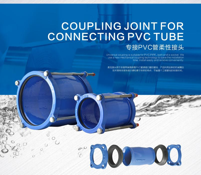
There is 5mm–10mm telescopic adjustment between socket. Another feature of the product is the range of connections. Because of the large diameter of the pipe connected to the product, the line is allowed to have a  $\pm$  3  $^{\circ}$  deviation when connecting the pipeline so that the normal movement of the pipe (such as ground subsidence, etc.). It can be used in the large bending radius pipeline caused the deviation.
