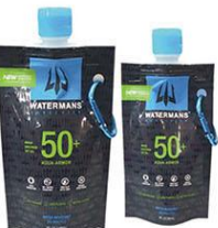
NO: 31 CONTENT: 3OZ & 5OZ MATERIAL: PET12/AL07/NY15/PE95 3OZ SIZE: 80MMX132MM+20MM 5OZ SIZE: 90MMX150MM+25MM SPOUT DIAMETER: 16MM
