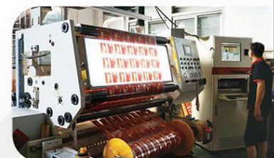
9 高速卧式全自动检品复卷机 High-speed rewinding inspection machine
