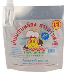
NO: 3 CONTENT: 4000ML MATERIAL FRONT: PET12/NY15/PE170 MATERIAL BACK: PET12+VMPET12+PE170 SIZE: 300MMX317MM+65MM SPOUT DIAMETER: 20MM
