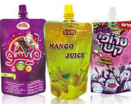
NO: 32 CONTENT: 250ML MATERIAL: PET12/AL07/NY15/PE90 SIZE: 100MMX165MM+30MMX2 SPOUT DIAMETER: 8.6MM
