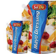
NO: 14 CONTENT: 250 & 500ML MATERIAL: PET12/AL07/NY15/LLDPE130 250ML SIZE: 115MM X 175MM + 30MM 500ML SIZE: 140MM X 230MM + 40MM SPOUT DIAMETER: 10MM
