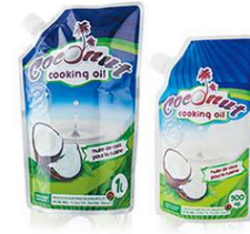
NO: 9 CONTENT: 1L & 500ML MATERIAL: PET12/AL07/NY15/LLDPE140 1L SIZE: 160MM X 250MM + 45MM 500ML SIZE: 125MM X 215MM + 35MM SPOUT DIAMETER: 15MM
