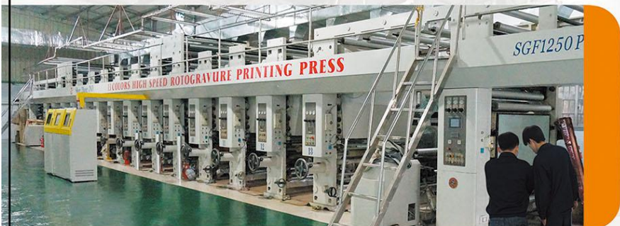
1 13 色高速印刷机 13-color high speed rotogravure printing machine
