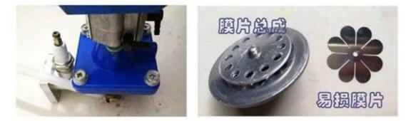
The elastic diaphragm is located under the four screws of the carburetor assembly. When the four screws are removed, you will see the right side of the diaphragm assembly. Open the middle of the screw, you can see a thin diaphragm. After the diaphragm is damaged, the smoke machine cannot start, and the damaged diaphragmneeds
