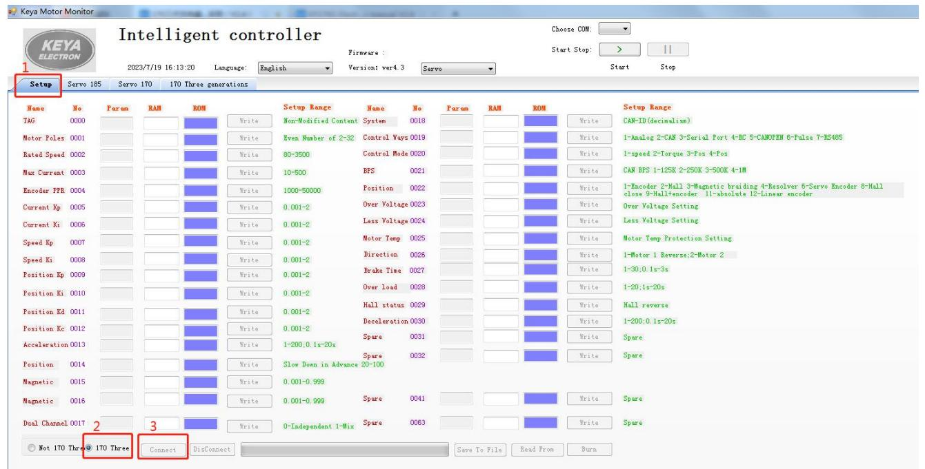
4.2.4 You can input data in the **RAM** column. The “Param” column means the motor parameters and ROM column shows the data reading from the E<sup>2</sup>ROM. In normal cases, the data in the three columns should be same. Due to the fast changes of software data, if data modification is needed, modify it quickly and click the “Write” button correspondingly.
