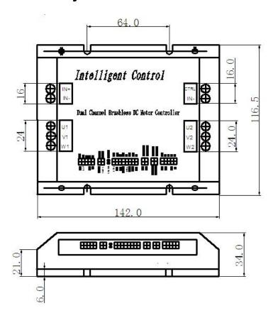
Note: The bottom of controller shell has  $4*\Phi5mm$  holes for installation and fixing, and installation can be conducted in the horizontal direction.
