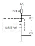
The controller provides 4-way digital output. The terminals are the MOS tube open-drain, the universal output amplitude is 24V 1A, and the maximum output is 40V 1A. In practical use, it is essential to connect a 10k pull-up resistor (as appropriate), as shown in the figure. For the digital output of every way, MOS tube breakover or turn-off can be chosen according to a preset event status.
