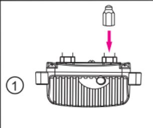
**Step 1:** Screw the metal prongs onto the trainer till the prongs are securely attached. Normally, they are assembled in the factory.
