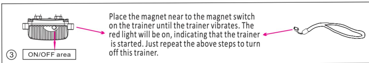
**Step 3:** To turn on/off the trainer, just make the magnet touch the magnet switch on the trainer until the trainer vibrates. The red and blue lights will flash once and the trainer will beep.
