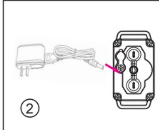
**Step 2:** Charge the trainer. Lift the small rubber tab on the trainer to access the charging port. Plug the wall charger into the wall socket and into the charging port of the trainer. A red led light will be visible on the trainer during the charging process.
