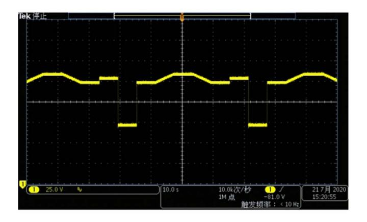
LV123 working range upper limit test waveform
