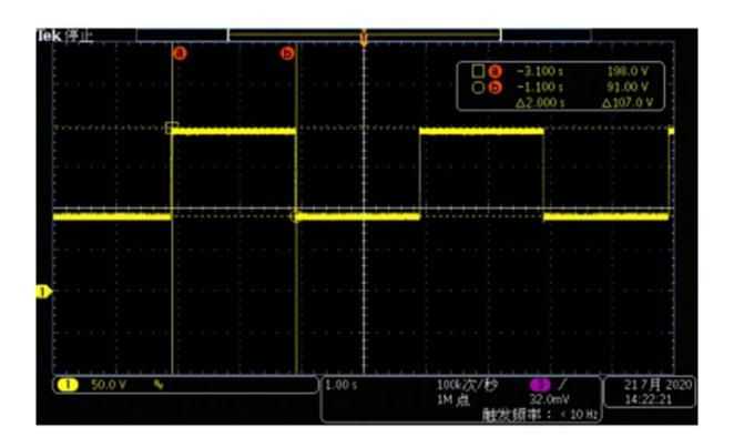
LV123 full-function working range test waveform
