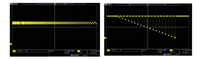
LV123 voltage ripple test waveform (ripple
