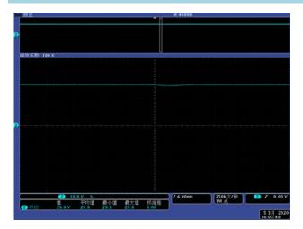
Output dynamic response waveform under  $10\% \sim 50\%$  load change
