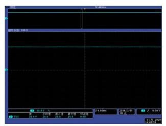
Output dynamic response waveform under 50% ~ 90% load change
