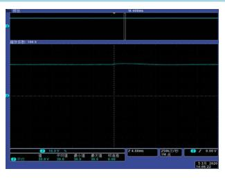
Output dynamic response waveform under 50% ~ 10% load change
