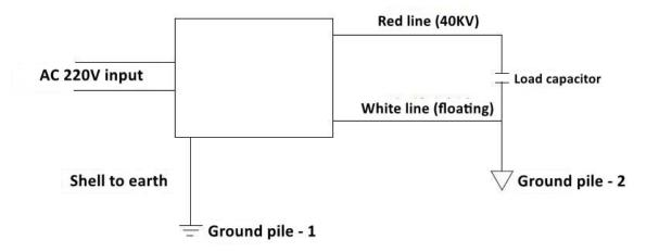
Product Description: Product grounding bolt on back panel connects to grounding pile 1, the black terminal on back panel connects to the floating white line, and the negative end of capacitance, that is, the pile 2 in the picture above.
