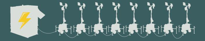
The main feature of the X7 Link light tower, up to 8 Link towers can be connected in series to a single power source, providing a high illumination area with reduced fuel consumption.
