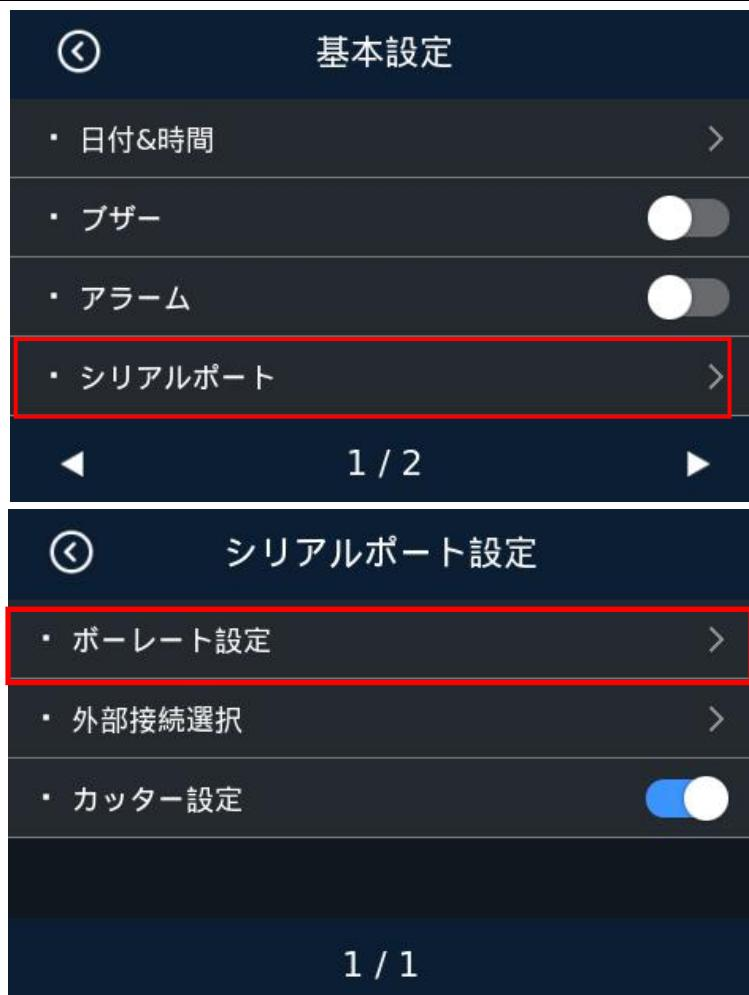
In the "ボーレート設定" selection interface, touch 9600 or 115200 to select the corresponding baud rate
