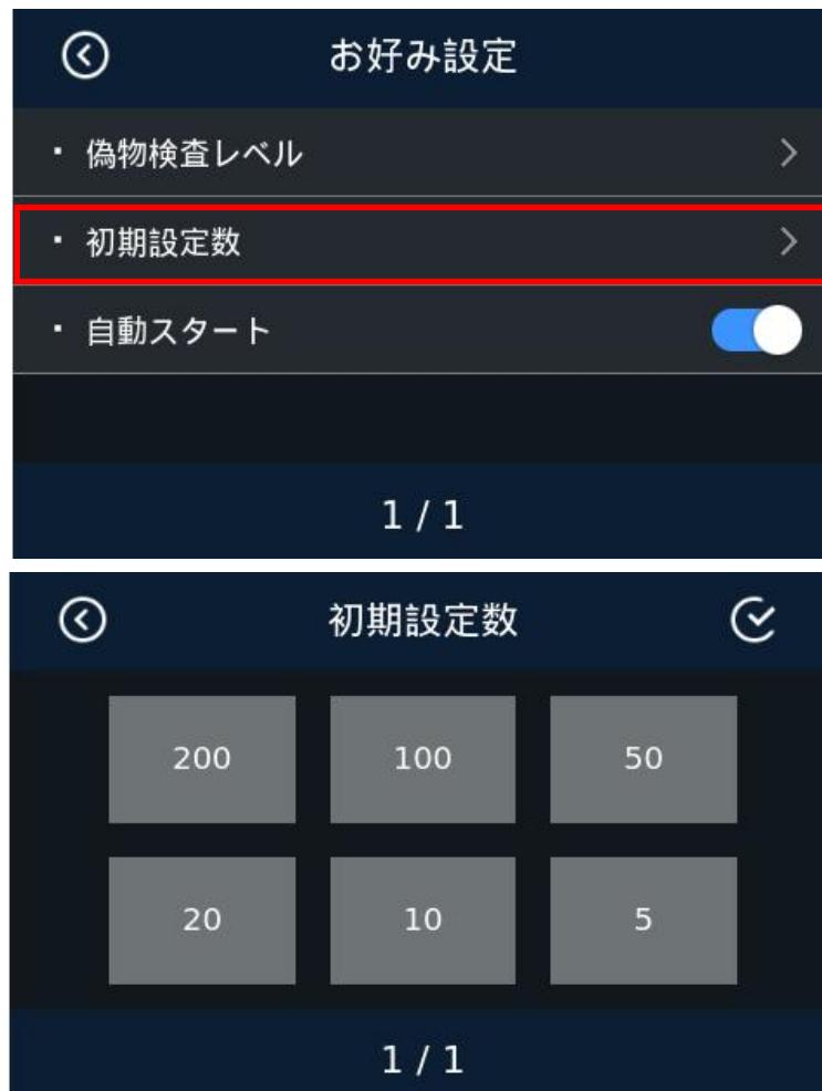
Touch the corresponding Batch number under this setting interface, directly enter the value to be changed (155 as shown in the figure below), and touch to confirm and exit. As shown in the following figure:
