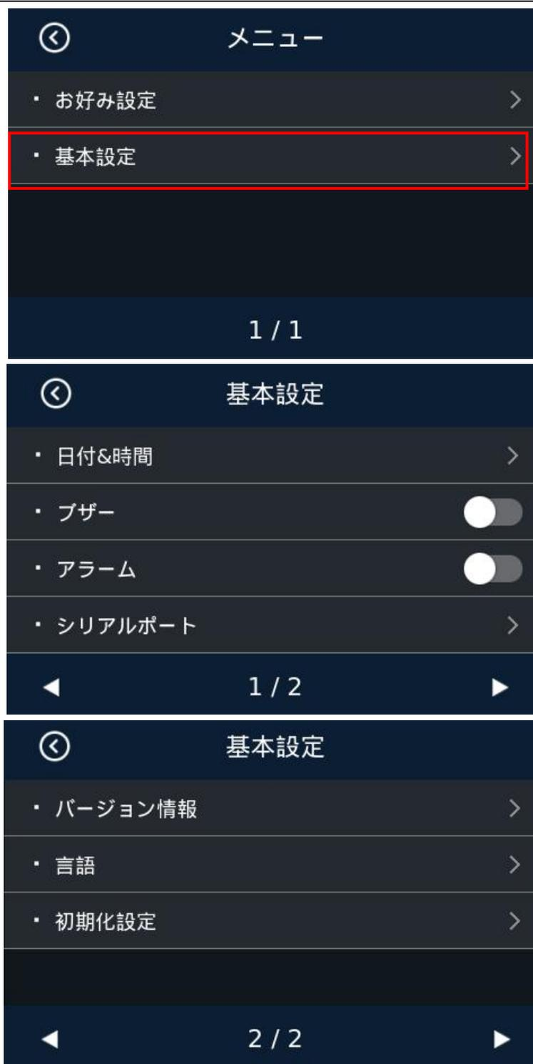
Under this interface, there are 7 items that can be checked or changed, including date/time, buzzer, alarm, serial port, version information, language, and factory settings. Touch left and right keys to check or change the items.
