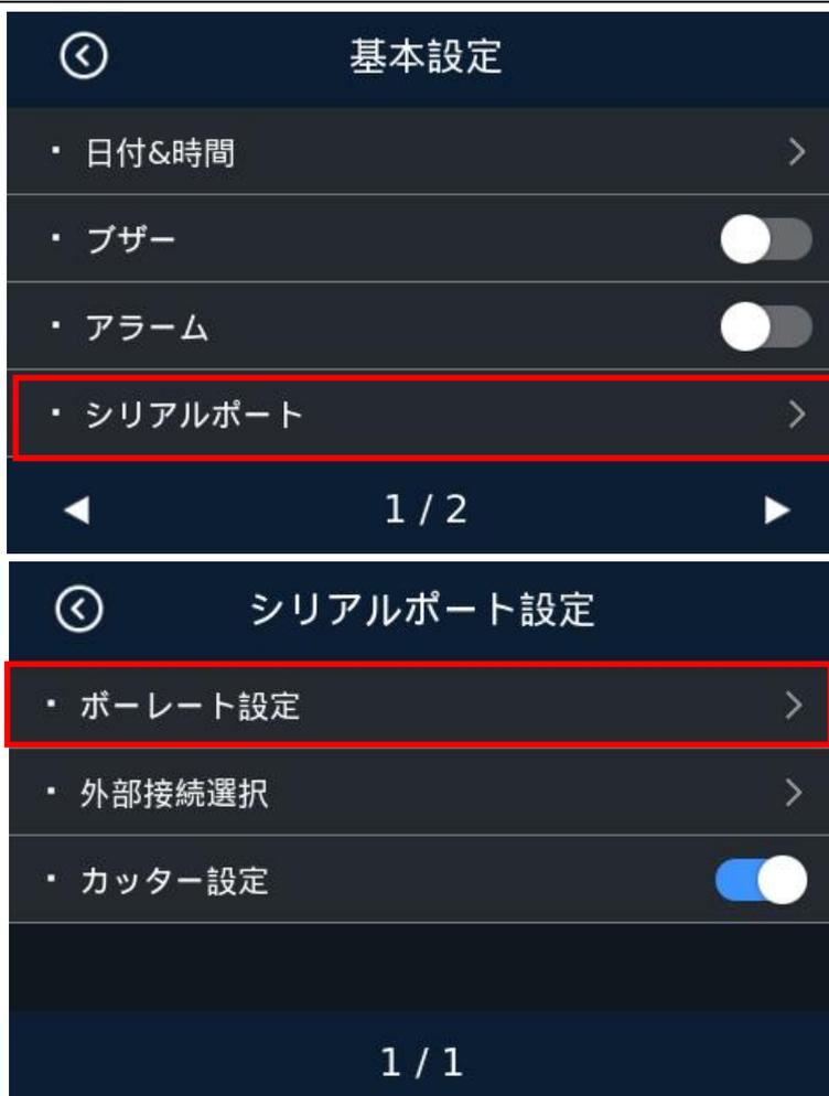
In the "ボーレート設定" selection interface, touch 9600 or 115200 to select the corresponding baud rate according to the actual situation of the external device. And click the
