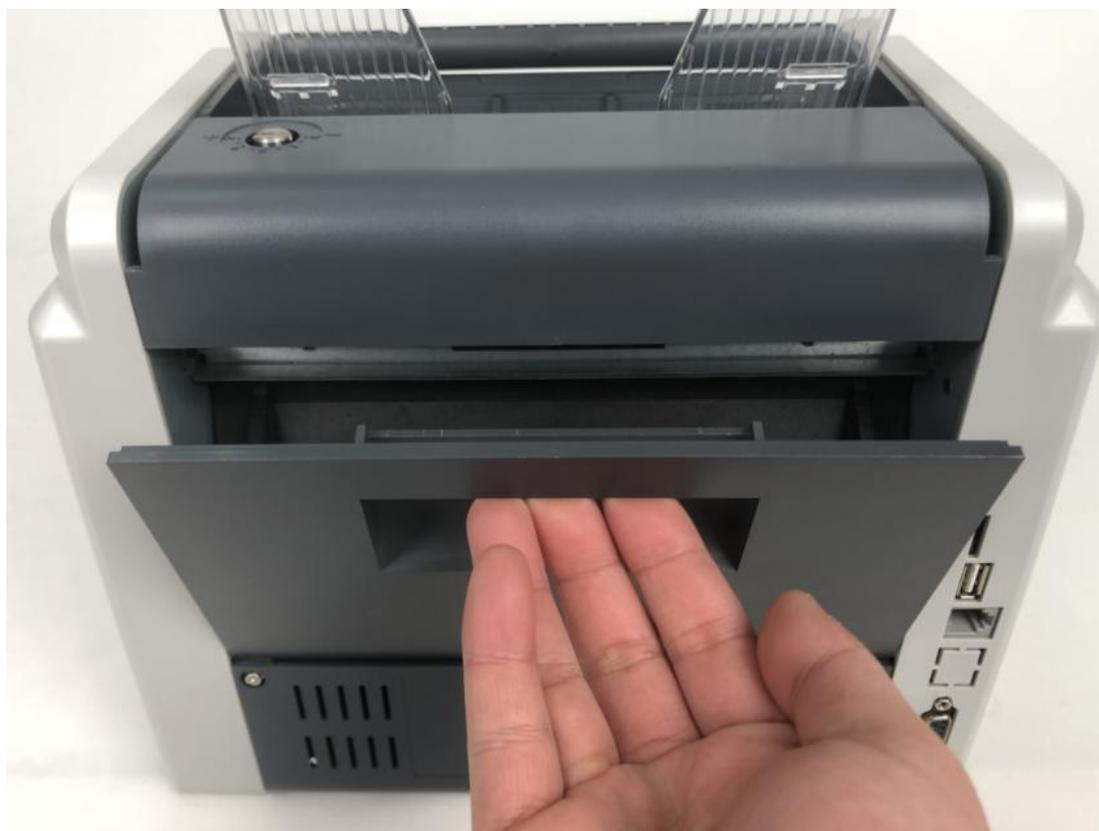
2) Clean the lower UV sensor and lower CIS with nylon brush respectively as shown in the following figure.
