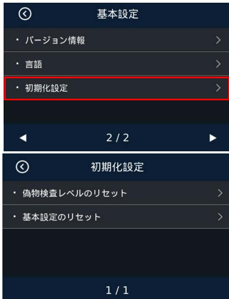
Touch **・偽物検査レベルのリセット** option. Click to restore all counterfeit detection levels to factory settings;
