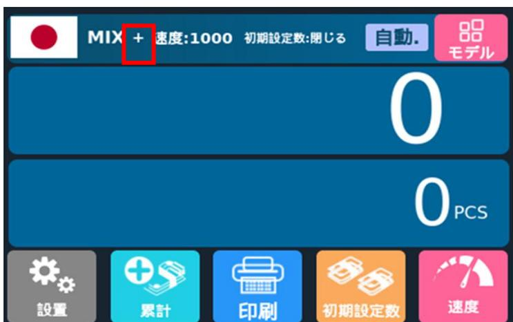
The accumulation function is enabled, and the symbol "+" appears
