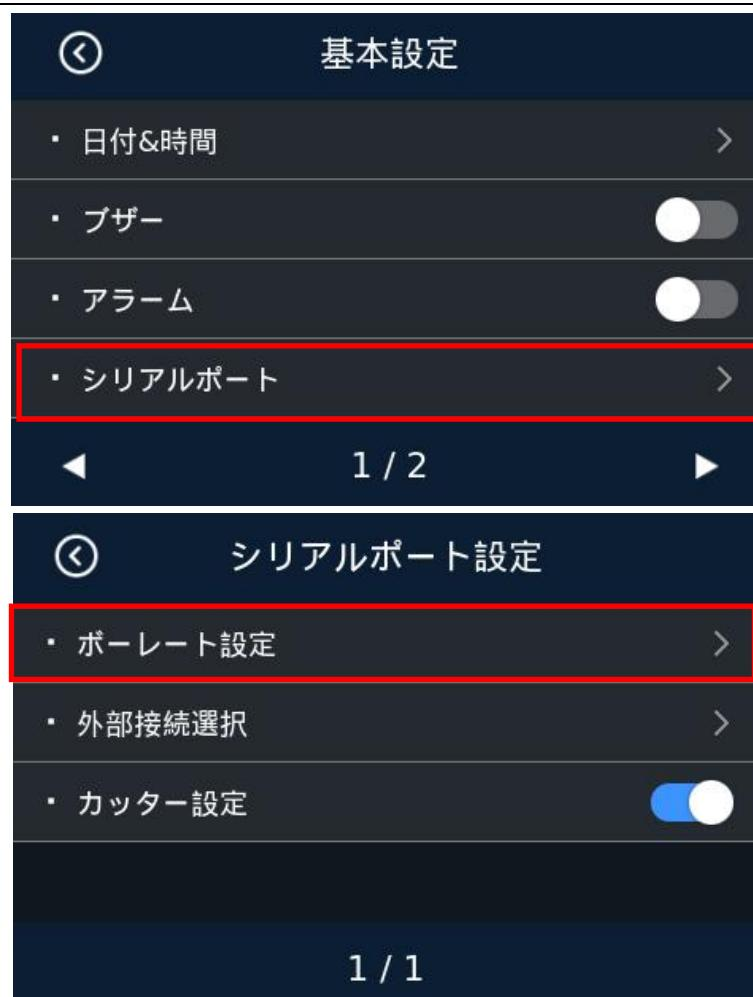
In the "ボーレート設定" selection interface, touch 9600 or 115200 to select the corresponding baud rate according to the actual situation of the external device. And click the key in the upper right corner to save. The machine will prompt you to restart.
