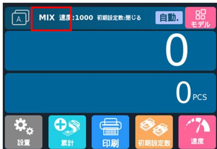
The accumulation function is off, and the symbol "+" does not appear.
