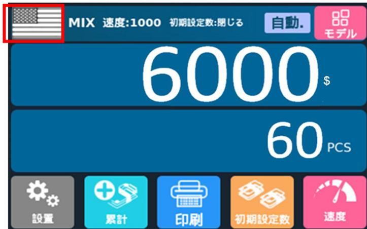
After the banknotes in the stacker are taken out, the machine will only display the total number and total amount of banknotes counted for the current time, and will not display the details of the previous yen banknotes, as shown in the following figure:
