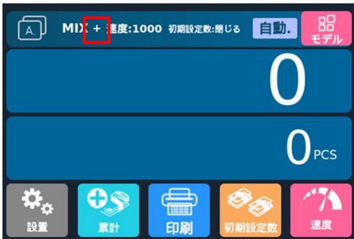
The interface of accumulation function on in the automatic mode
