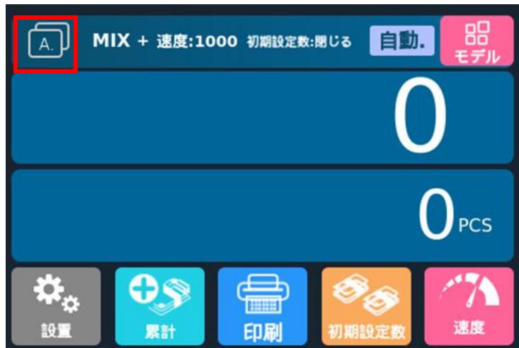
In the automatic recognition mode, there is only one MIX Counting Mode, and the display of machine counting information will be different when the accumulation function is off and on.
