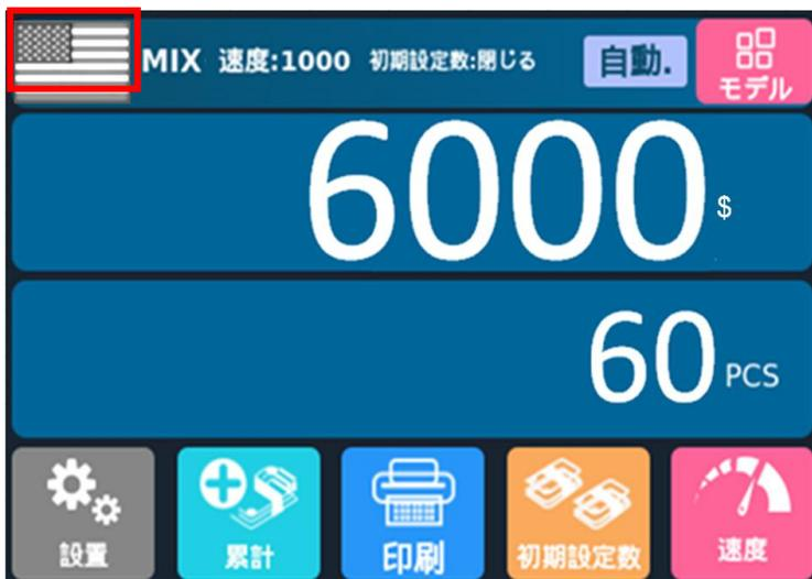
After the banknotes in the stacker are taken out, the machine will count and accumulate the details of the previous and current counting, and the following interface will appear:
