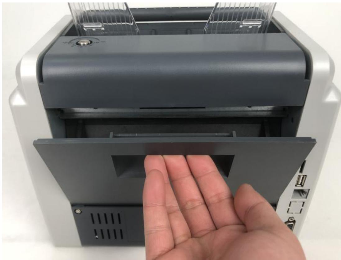
2) Clean the lower UV sensor and lower CIS with nylon brush respectively as shown in the following figure.
