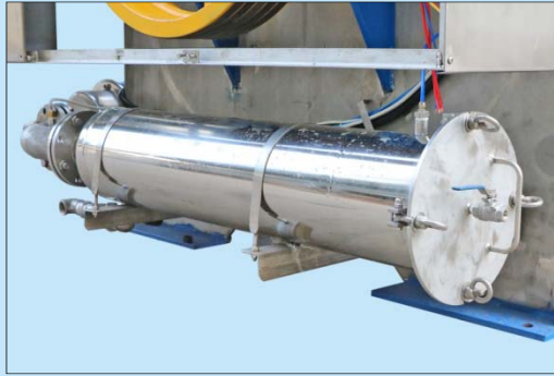
循環運水配合過濾系統 Circulating Water System Combined With Filtration System
