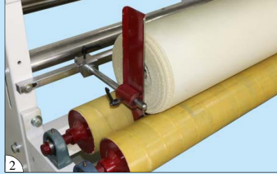
2 捲布擋板，能降低捲布時布卷左右擺動的範圍 Winding baffle can limit the fabric swing range during winding
