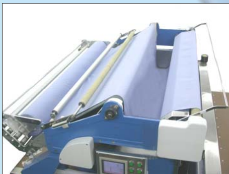
“U”型松布功能，無張力拉布 “U” Type Fabric Loosening for Tension Free Cloth Laying
