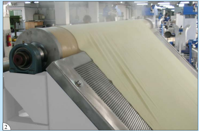
2. 前方噴蒸汽預縮區 Front steam spraying pre-shrinking area
