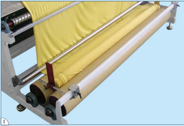
1. 托布軸連展布系統 Fabric supporting shaft with fabric spreading system
