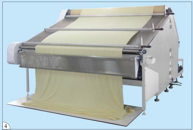
4. 搖臂式折疊系統 Swing arm type folding system
