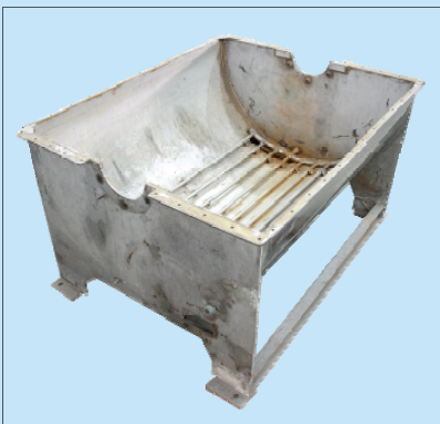
蒸汽間接加溫內部管道圖(NS-2701系列) Indirect heating device (NS-2701 series)
