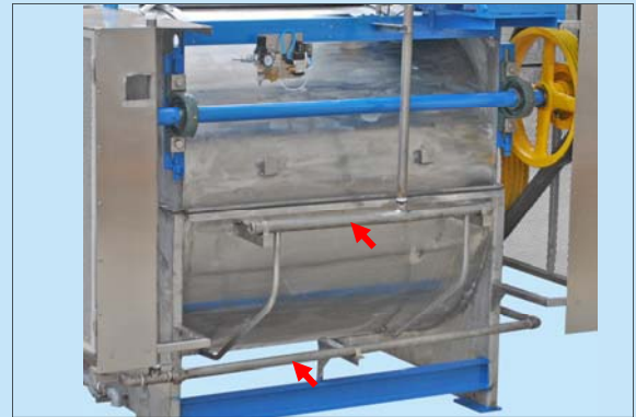
蒸汽直接加溫與間接加溫裝置(NS-2701-200) Direct and indirect steam heating device(NS-2701-200)
