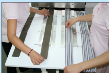
粘褲襠 Waistband and tape fusing
