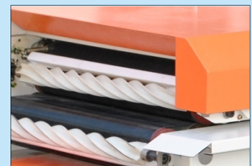
特殊的清潔、收料系統 Special designed cleaning and material collecting system
