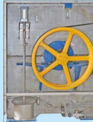
O-I-09-2 另增氣動排水控制系統(程控)-Ø8" Additional Pneumatic Water Draining Control System(program control)-Ø8"
