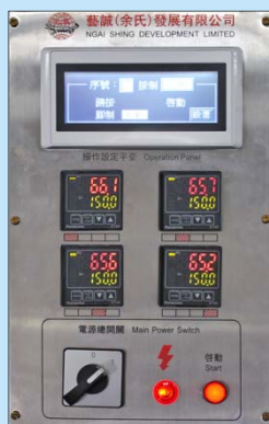
PLC + 觸摸屏 PLC + Touch screen
