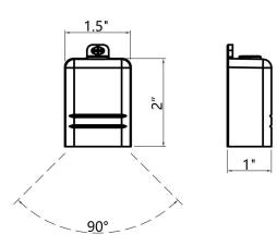
Model: MWL-LSS01 Type: Low Voltage LED Color Temp: 2700k/3000k Operating Voltage: 9-15v AC/DC Wattage:3w Beam Angle: 90° Wire Lead: 4ft Lumen: 270LM CRI: 80 Efficiency: 80 Weight: 0.17 KGS Waterproof Grade: IP67 Material: Heavy Duty Cast Brass
