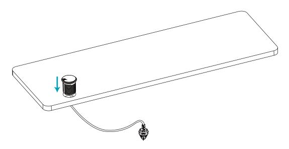
**3** Screw the installation accessroy make the socket fix with the surface bottom.
