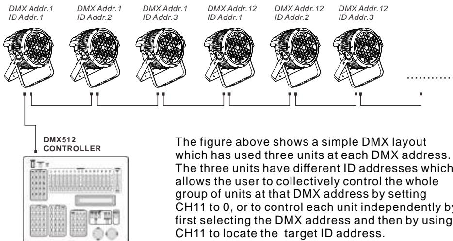
The figure above shows a simple DMX layout which has used three units at each DMX address. The three units have different ID addresses which allows the user to collectively control the whole group of units at that DMX address by setting CH11 to 0, or to control each unit independently by first selecting the DMX address and then by using CH11 to locate the target ID address.
