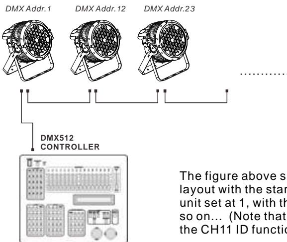
The figure above shows a simple DMX512 layout with the starting address of the first unit set at 1, with the second set at 12 and so on... (Note that when used in this way, the CH11 ID function must be inactive (CH11=0))
