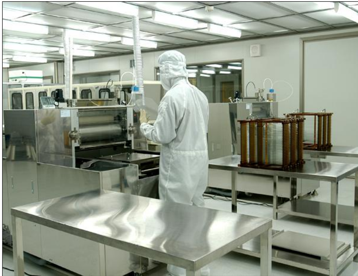
PI COATING & PREBAKING MANUFACTURING WORKSHOP(CLASS 100)
