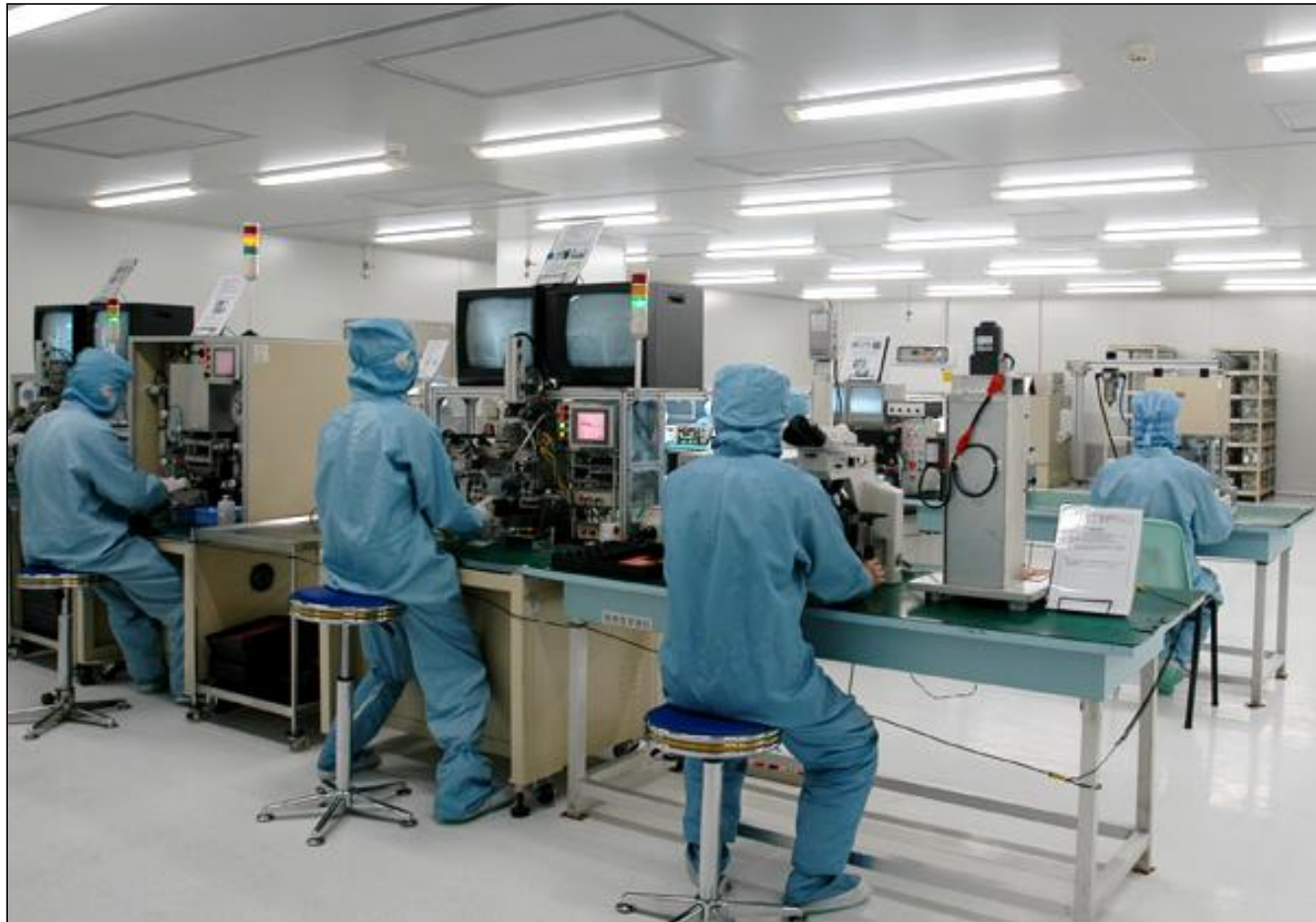
COG&TAB BONDING MANUFACTURING WORKSHOP WITH ANTI-STATIC FLOOR (CLASS 1000)
