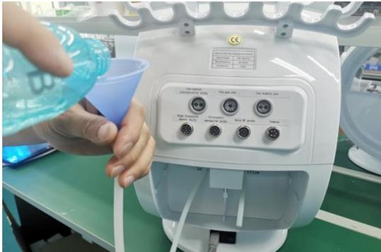
1) D solution bottle installation and disassembly Disassembly: Fasten the groove of the solution bottle with your hands and pull it back to complete the disassembly.
