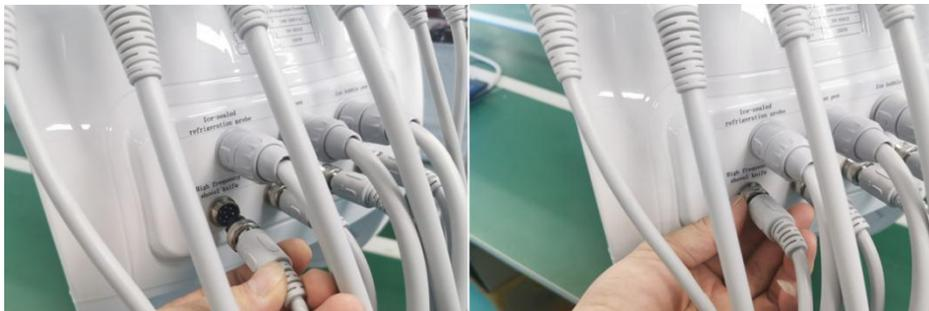
3) Corresponding connection hole for each hand tool probe
