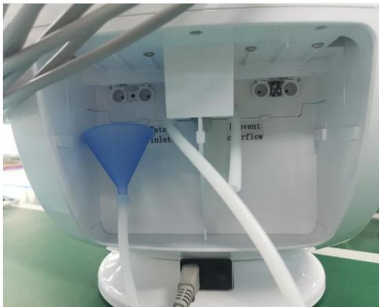
The third step: Pour purified water (must be pure water) into the water filling port, and when the water is full, it will flow out from the overflow port, and the filling is completed
