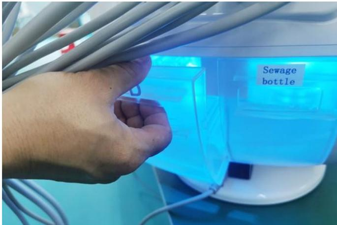
4) Removal and installation of sewage bottle
