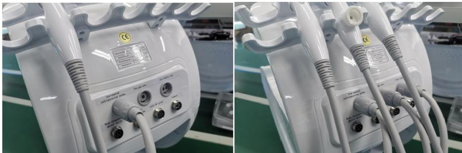
2) Installation of high-frequency shoveling knife, ultrasonic lead-in head, golden radio frequency head, and camera
