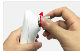
Install Probe (FIG2)
