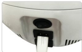
Connect the handle cord( FIG. 4 )
