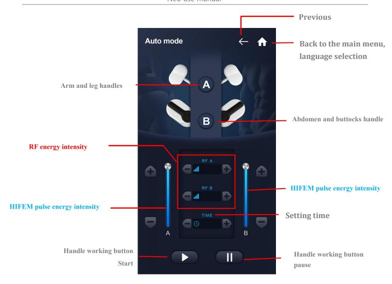
$2\sqrt{1}$  The AB handle can be selected independently, the strength/time of the handle can be adjusted according to different customers, and the start/stop button can be clicked to operate
