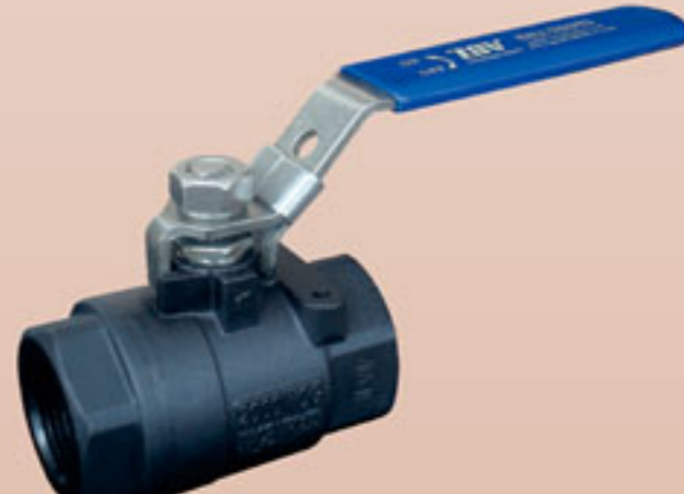
2004WC SERIES 2000PSI 2-PC BALL VALVE FULL PORT SIZE: 1/4"-2" SEAL WELDED API607
