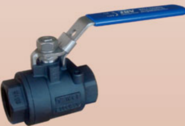
2006WC SERIES 2000PSI 2-PC BALL VALVE FULL PORT SIZE: 1/4"-2" SEAL WELDED
