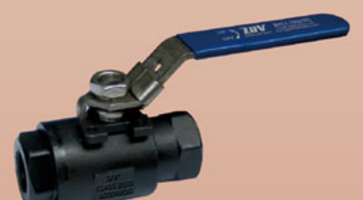
1532C SERIES 1500PSI 3-PC BALL VALVE REDUCED PORT SIZE: 1/4"-2" API607
