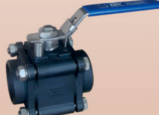
1531C SERIES 2000PSI 3-PC BALL VALVE REDUCED PORT / FULL PORT SIZE: 1/4"-1" 2000WOG 1 1/4"-2" 1500WOG
