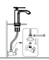
4. the two water hose connection on the angle valve faucet body. "Red" and "blue" in accordance with the dot on the handle faucet tips are connected
