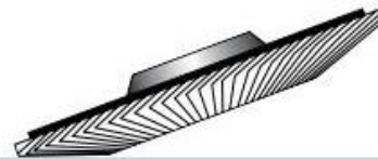
GRIND AT STEEPER ANGLES: 15° - 25°
