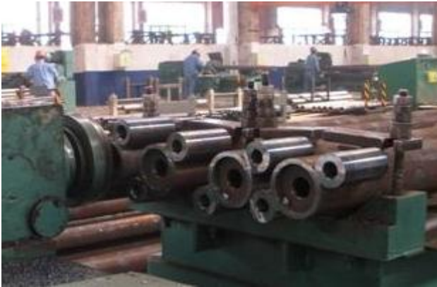
Double-sided milling process
