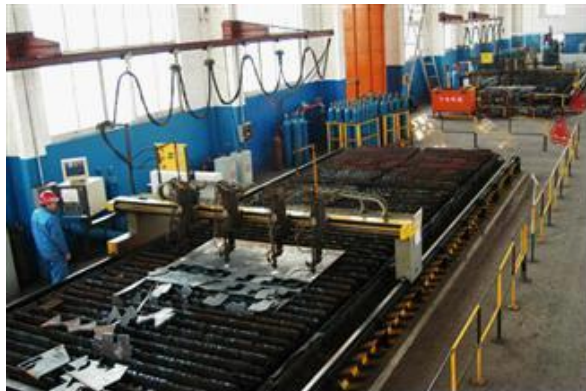
CNC flame cutting
