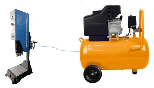
B.ultrasonic welder+hose1+hose reducer+hose2+air compressor
