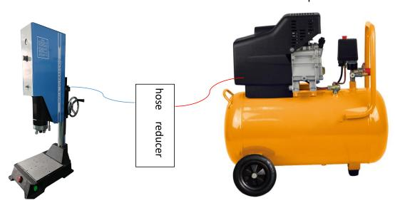
4) The ultrasonic welder requires 220V supply. If the user do not have 220V supply on site,
