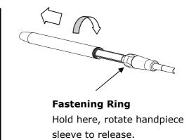
To take off the handpiece sleeve, please hold the fastening ring, and rotate the sleeve counterclockwise from handpiece tubing assembly. **Note: Avoid rotate or twist the handpiece tubing.**
