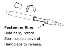
To take off the Sterilizable sleeve of handpiece, please hold the fastening ring, and rotate the sleeve counterclockwise from MS handpiece cable set assembly. **Note: Avoid rotate or twist the MS handpiece Cable .**
