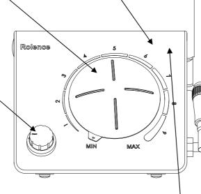
AC Power Indicator Light Illuminates when the system is switched on.
