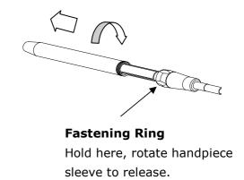
To take off the handpiece sleeve, please hold the fastening ring, and rotate the sleeve counterclockwise from MS handpiece cable set assembly. **Note: Avoid rotate or twist the MS handpiece cable.**
