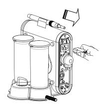
2. Turn the pump set moderately in the direction of counterclockwise at about 30 degree. Then pull out the complete used pump set with tubing.
