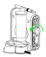
3. Reverse the procedure above, replace with a new tubing pump set.
