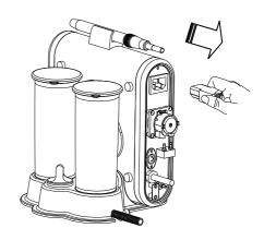
2. Turn the pump set moderately in the direction of counterclockwise at about 30 degree. Then pull out the complete used pump set with tubing.
