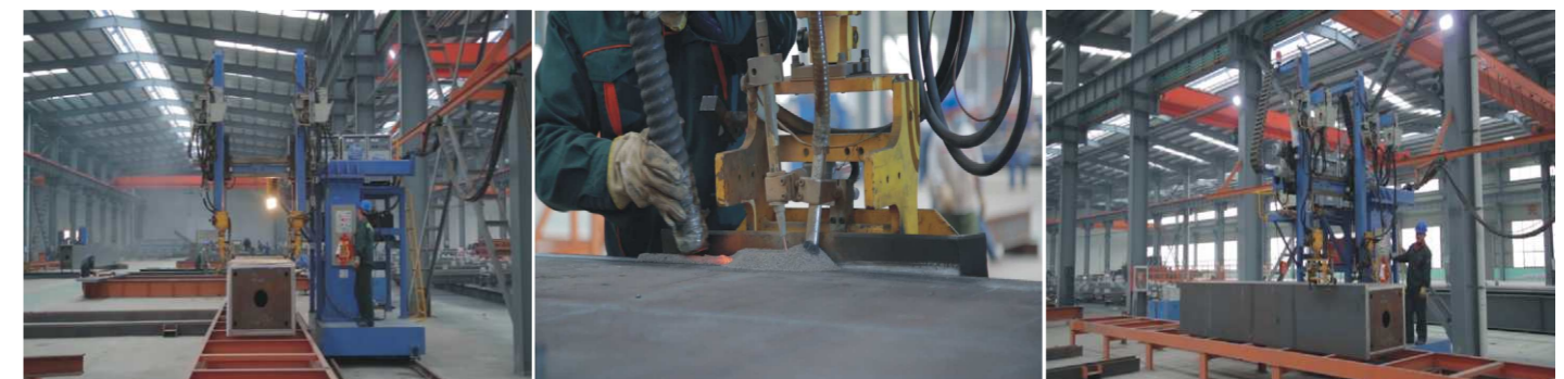
Triple wires with triple arc ( 2DC+AC )
