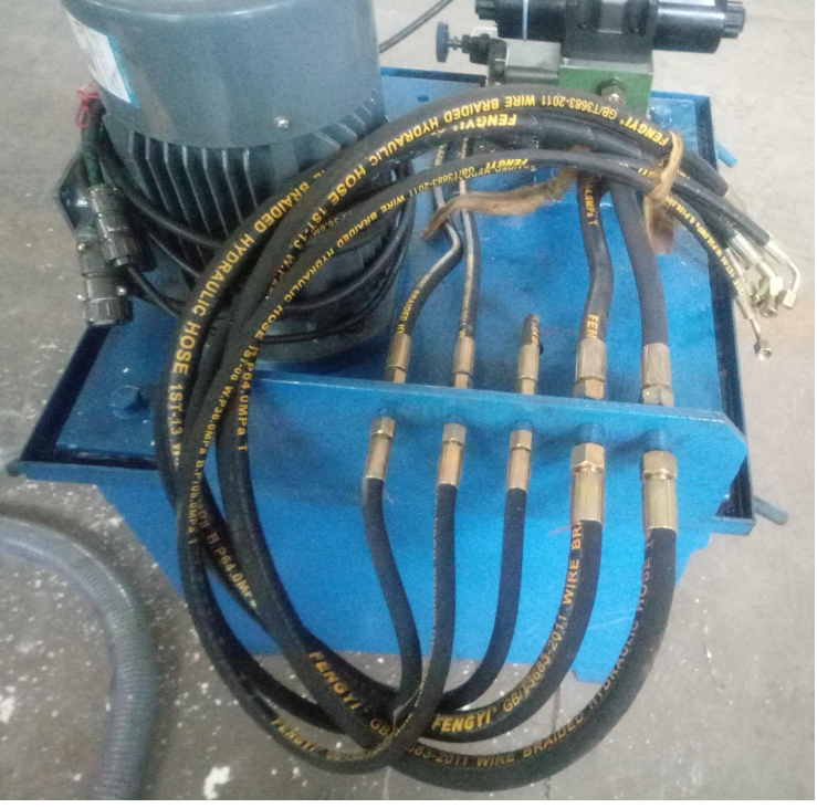
Hydraulic pump station
