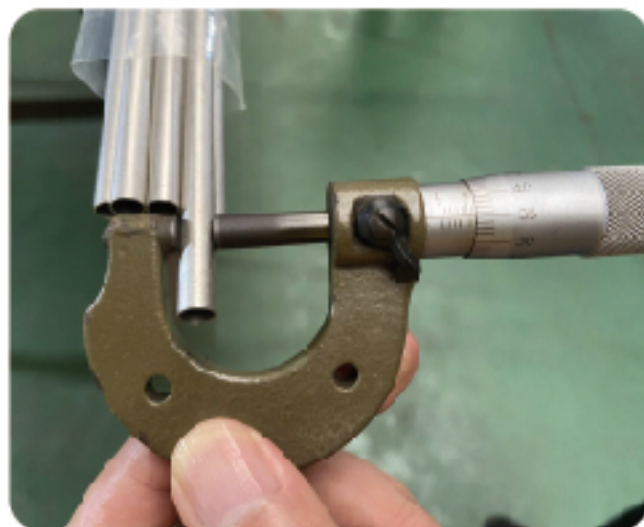
Capillary tube Min. O.D. 1.5mm
